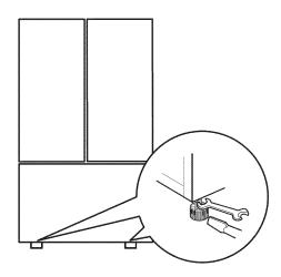
**NOTE:** Having someone push backward against the top of the refrigerator takes some weight off of the leveling legs. This makes it easier to adjust the legs.
